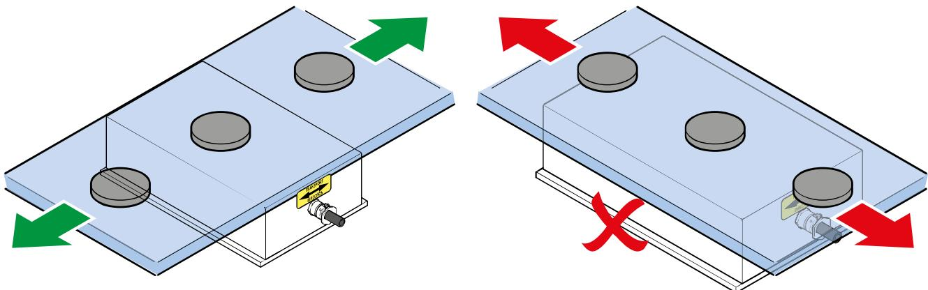
The material to be demagnetized must be guided as close as possible, and as evenly as possible, across the device's contact surface.
