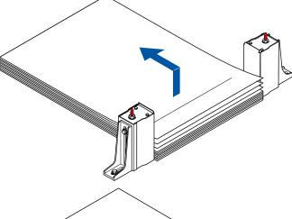
For a stack of **large steel sheets**, position the devices at the corners.
