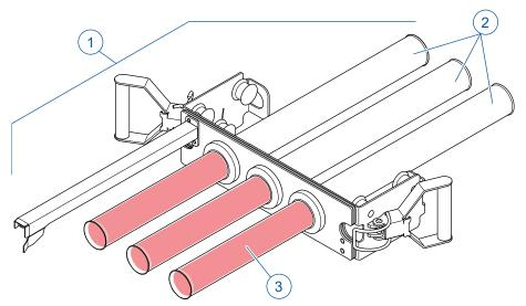
The magnet unit [1] comprises a magnet drawer with 2 or multiple pneumatic magnetic bars [2].
