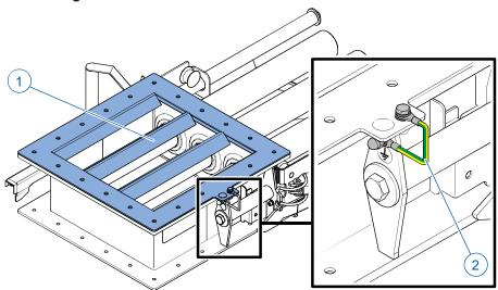
A deflector grille [1] is optionally available to ensure that all particles in the product flow make contact with the magnetic bars or pass them very closely. If the device is supplied with a deflector grille, it will also have an earth cable [2]. This also applies to devices supplied with adapter pieces.
