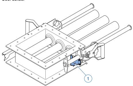
A door sensor (safety sensor, e.g. Steute Ex HS Si 4) can be optionally fitted to the mounting bracket [1] that detects when the magnet unit is open (removed) or closed. Because this sensor is used for detection, rather than a safety-related function, it is not necessary to connect it to a special safety relay for contactless sensors, which additionally feature current limitation and short-circuit detection.
