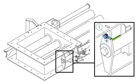
In order to prevent the occurrence and build-up of static electricity, ensure that there is a metal bridge between the magnetic device/product channel and the installation. The installation must be earthed when complete.
