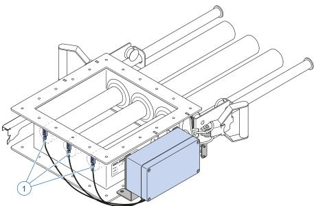
As an option, detection sensors [1] can be placed on the outside of the product channel to detect whether the magnet unit is positioned fully in the product channel. The detection sensors can be connected to a central controller. When the detection sensors detect all magnetic bars fully in the product channel, a signal is sent to the (central) controller so that production can commence.
