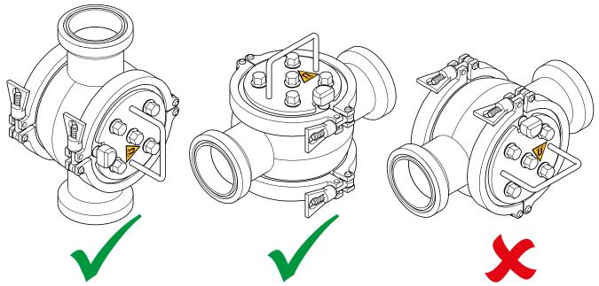
NEVER install the device with both connections and the magnet unit positioned horizontally, due to pipe drainage concerns.
