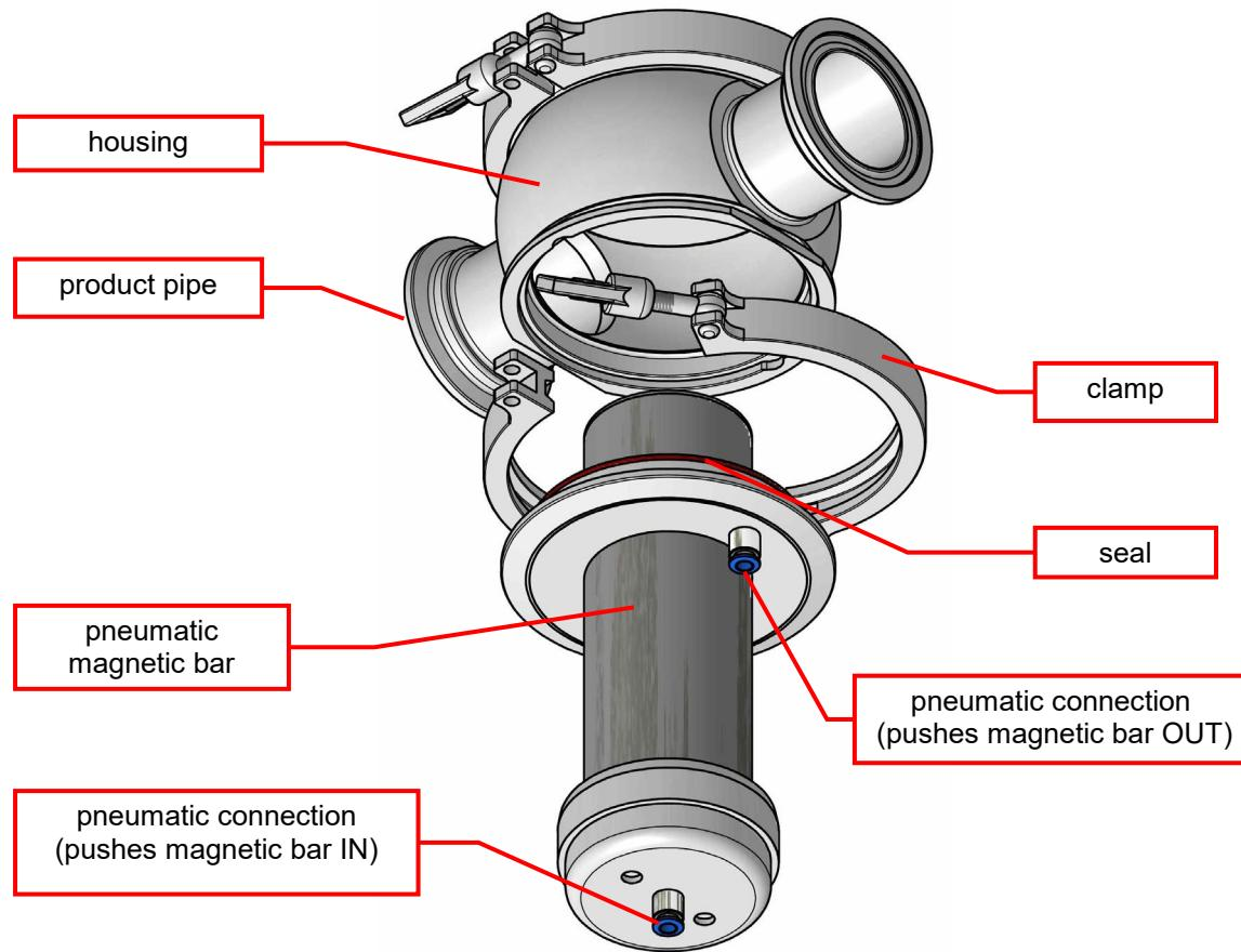
The function of the device is to catch ferromagnetic contamination from the product stream.
