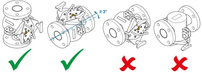
• The devices are available with various EN1092-1 flanges and couplings. Follow the installation instructions in accordance with the relevant standards for the flanges and couplings to install the device in your installation. Misalignment or loose mounting can cause leakage.
