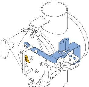
The device can be fitted with a padlock. This prevents removal of the magnet unit from the housing.
