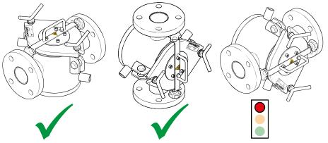
• Install the device in the horizontal orientation with the magnet unit at the top. If this is not possible, bear in mind when opening the lid that residue will run out during maintenance work (see figure).
