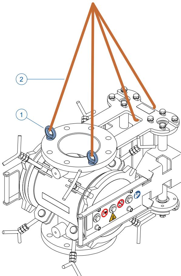
Lift the unit evenly out of the crate as shown. Use a hoisting unit that supports the device.
