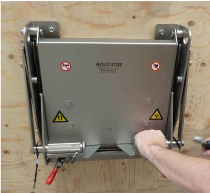
Once the chute magnet is mounted against the product chute, remove the tie-wraps.
