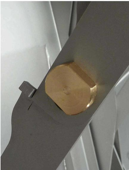
When closing the magnet, pull the magnet unit open slightly (this releases the arm from the metal notch). Then turn both the metal rods slightly upwards to fold the arms. Keep in mind that the tubes operate independently, so two-handed operation is required.
